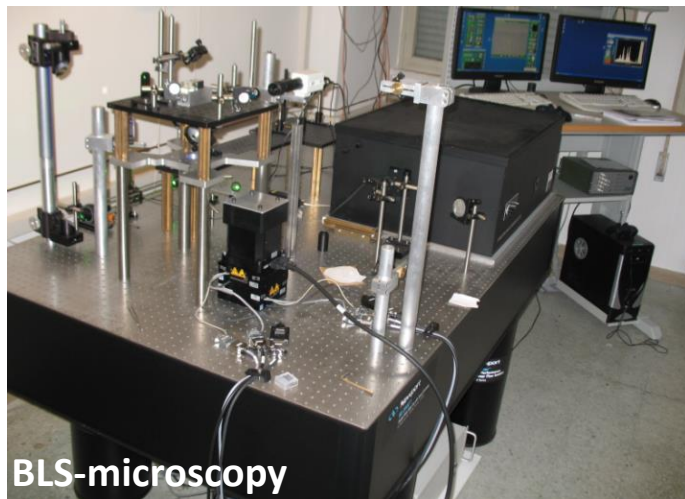
(inelastic scattering of photons by spin waves "magnons")
